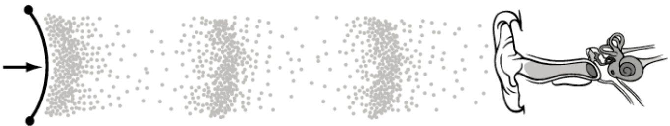
Figure 2.1 A vibrating string produces a series of compressions and rarefactions that are received by the ear, coded as neural impulses, and sent to the brain.
