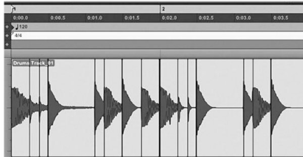
Figure 2.15 The results of transient analysis. The vertical lines indicate identified beats. (Screenshot is provided courtesy of Avid Technology, Inc.)
